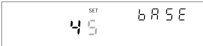
Base Channel Number display for setting the BCN 10s digits (for example, 45)
